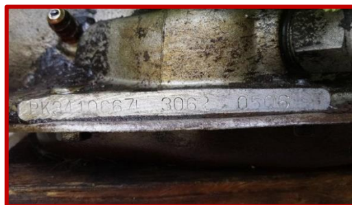
A number etched or cast into the transmission case.
