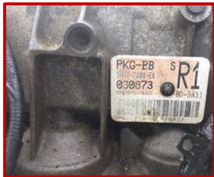
A steel tag riveted to the transmission case
